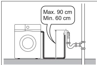
The end of the drain hose must always be ventilated, i.e. the inside diameter of the drain pipe must be larger than the outside diameter of the drain hose.
