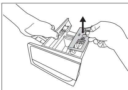
Flush it out under a tap to remove any traces of accumulated powder.
