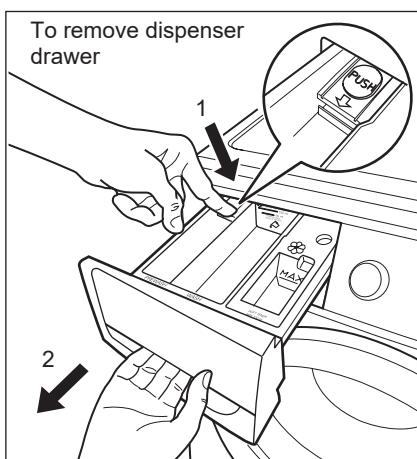
To aid cleaning, the top part of the additive compartment should be removed.
