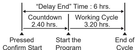
After selecting Delay End time, press “Start/Pause” and “Confirm Start” touchpad to start the program. Machine will then countdown and update time on the display every hours until it reaches the starting point of the wash cycle.
