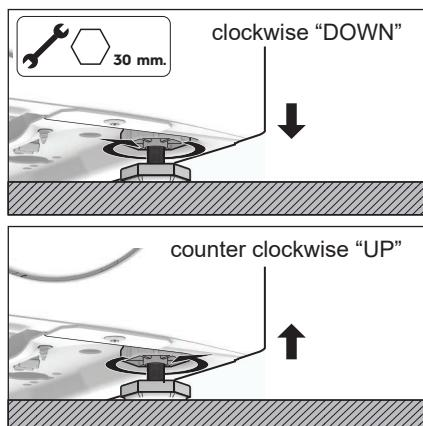
When the washing machine is levelled, try to rock it from corner to corner. If it does rock, adjust the legs again until it is levelled and does not rock.
