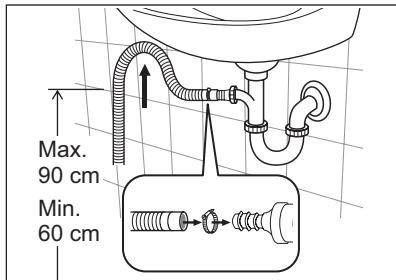
Push the drain hose onto the spigot and secure with a clip, ensure a loop is formed in the drain hose to prevent waste from the sink entering the appliance.
