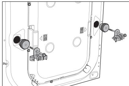
**Transit bolts must be removed before using the appliance.**
