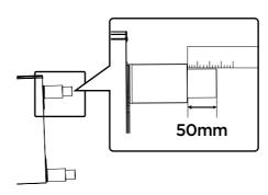
For a 900mm height kitchen bench top, adjust the lower half of the feet to measure 50mm as shown in the illustration.
