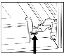
Press the locking tab down for removing the door.
