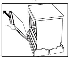
Tilt and carefully lay the appliance on its back to gain access to the installation point for the screw in feet.
