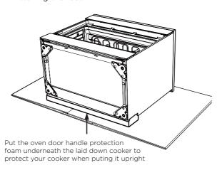
Install the four supplied feet via the four installation points. Make sure that each foot is securely fastened.
