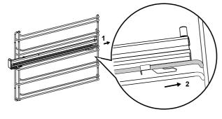
3. Push slide front clip over wire until secured
