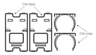
Assemble the clip snap onto the base.
