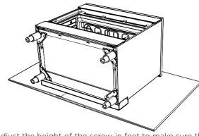
Adjust the height of the screw-in feet to make sure the hob surface is 10mm above the bench when appliance is upright.
