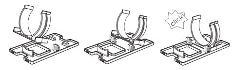
Press in both assembled clip modules into the kick panel in the orientation as shown below.
