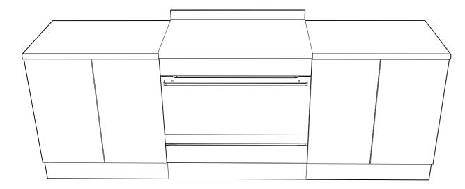
The slot-in type installation use the appliance as supplied. The appliance can be mounted on a plinth. This enables a continuous cupboard kickboard to be installed, giving a more integrated appearance. There is no clearance requirement between oven and adjacent side cabinets.
