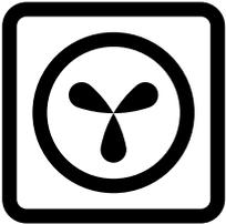
Heat comes from the gas “base heat” burner which is then circulated by the fan. This fan circulates the hot air around the oven cavity so that you can put your food in different places in the oven and still cook them at the same time.
