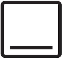
Heat comes from the gas “base heat” burner below the food. The bottom burner is below the floor of the oven which is controlled by the thermostat and will turn on and off to maintain the set temperature.
