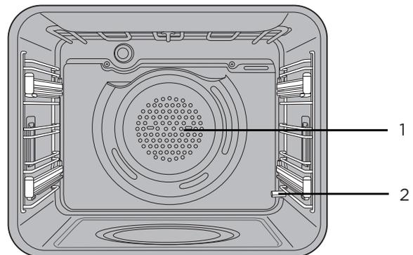
1. Steam outlet. This is where steam is injected into the oven, which is behind the fan cover.
