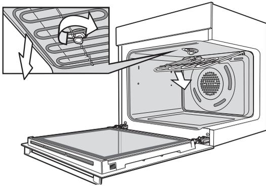
Retaining clips models - The upper grill element is secured with 2 clips which can be removed to help clean the oven cavity ceiling. To disengage the clips, push the edge of the clips towards back of the oven as shown below. After cleaning raise the grill element and secure clips back in position.
