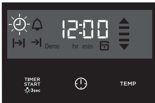
When power is supplied to the oven the clock icon will be displayed. Along with the clock symbol the '12' will be flashing. This indicates that 'hour' portion of the time is ready to be changed.
