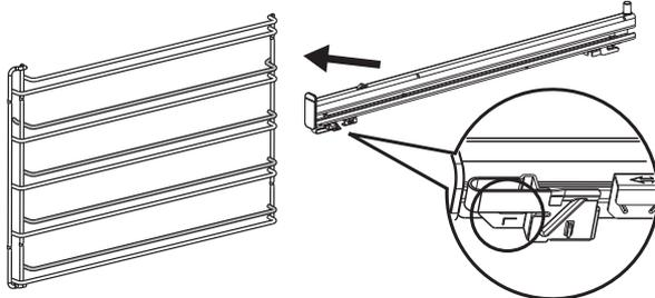
2. The shaded wires indicate the wire the slide can be mounted on. Fit slide rear clips to the rear of wire at an angle as shown below.
