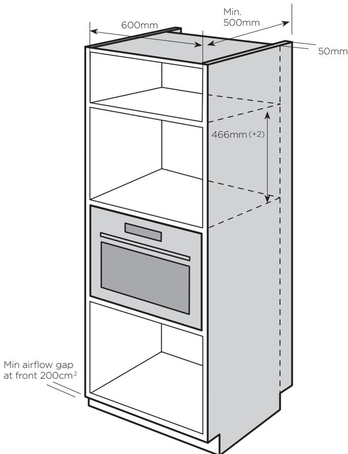
A 50mm ventilation gap must be left between the built-in cabinetry and wall with no back panelling on the cabinet housing the microwave oven. A minimum ventilation gap of 3.5mm must be left between the bottom of the front trim and adjacent shelf/cupboard.
