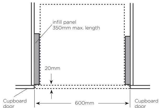
Infill panels are recessed 20mm from the external cabinet door to accommodate flush fit.
