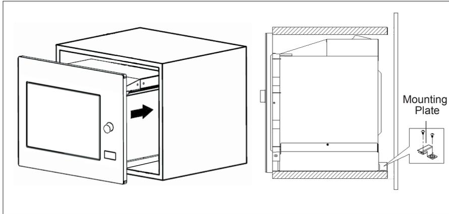
2. Open the door and fix the oven to the cabinet with Screw B, at the installation hole. Then fix the Trim-kit plastic cover to the installation hole.
