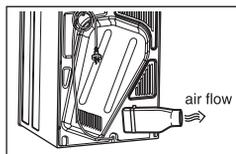
Inlet and outlet points need clear airflow to prevent overheating, so ensure there is adequate ventilation. (i.e. open window or external door.)
