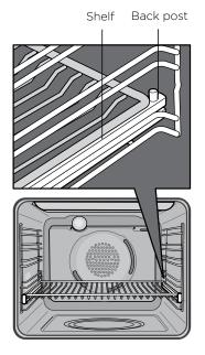
Drop the front of the shelf or tray onto the slide ensuring it sits behind the front post of the slide.
