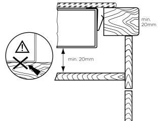
It is recommended to centre the bench cutout with equal distance front and back as shown but the product has also been certified to be installed with no clearance between the rear edge of the cooktop glass and rear wall if required. In doing so installers still need to leave sufficient clearance to take into account that the glass dimensions are larger than the cut out
