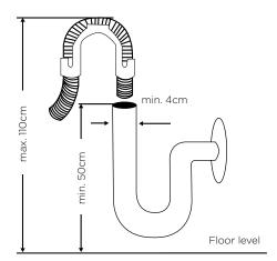
The water drain hose can be connected either directly to the water drain hole or to the sink outlet spigot. Using a special bent pipe (if available), the water can be drained directly into the sink via hooking the bent pipe over the edge of the sink. This connection should be at a minimum of 50cm and at a maximum of 110cm from the floor.
