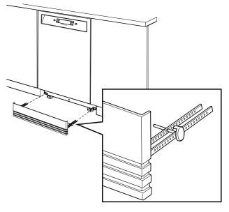
When installing the adjustable plinth to undercounter height cabinets 870-920mm, kit #52075772 must be purchased.
