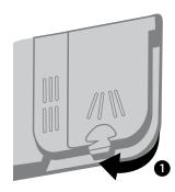
Push the latch to open the detergent container as shown in the image **①**. Detergent pod has level lines inside, measure the detergent amount using these lines. Detergent pod can take a total of 40cm³ detergent.
