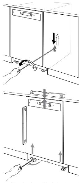
Open the dishwasher door and fix the brackets with the screws provided.
