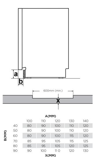
When installing the adjustable plinth to standard undercounter height cabinets (820-870mm), attach the 2 adjusting brackets to the metal plinth with the screws provided.
