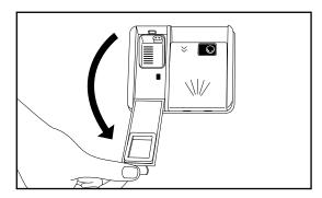
Fill the compartment with rinse aid until MAX level and then close the cap.
