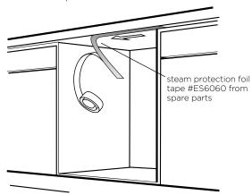
2. Adjust the dishwasher feet according to the slope of the floor then carefully slide the dishwasher into the cavity.
