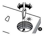
The rinse aid level adjuster can be set to a position between 1 and 6. Factory setting for rinse aid is the position 3. You need to increase the degree of the adjuster if water stains form on your dishes after a wash, whereas you need to decrease the degree if a blue stains left when wiped by hand. 3
