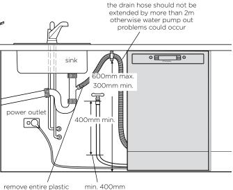
remove entire plastic membrane from sink trap spigot and fit drain hose to spigot with clamp min. 400mm straight section
