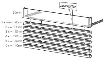
Use the 2 plastic locking pins to set the position of the plinth assembly.
