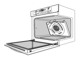
Removing and replacing the catalytic fan baffle (where fitted)
