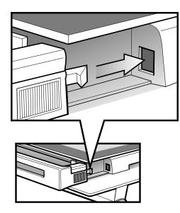
• Push the middle of the trim down to ensure it is straight and firm against the glass panel.
