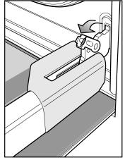
• Gently close the oven door until it stops on the locating tabs. The door is now ready for dismantling.
