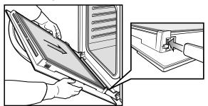
• Open the door fully to access the hinges then rotate the 'stirrups' (see image below) until they lock into the hook. The oven door may now be closed.
