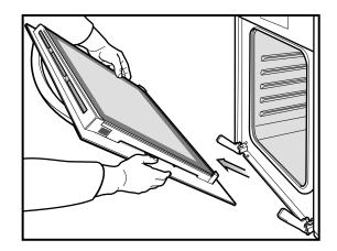
• Lay the oven door with the outer side facing downwards on something soft and flat (for example a blanket on a kitchen table) to prevent scratches.
