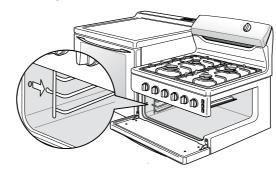
The door on your cooker is designed to allow cool air to pass up through the middle and out through the vent in the top of the door (see diagram below).
